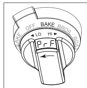
Figure 3-45. Turn and Hold Control Knob to Left until “PrF” is Displayed
